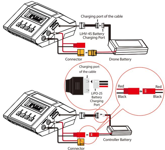
1. Before charging, check that the terminals and wires of the battery pack are not damaged.
