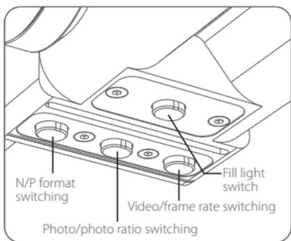
**Fill light switch:** Short press to turn it ON/OFF
