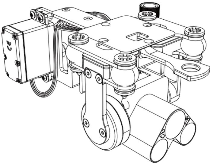
PL4-HS – Low light payload release for SplashDrone 3+. For low-light and night-time payload release, the PL4 utilizes a high-sensitivity sensor and dual LED spotlights to return colour HD images in near darkness. Get live as well as recorded video footage from the drone and accurately locate your target zone at night before remotely dropping your baits. Add the optional burley dry chum release system takes your night fishing to the next level.
